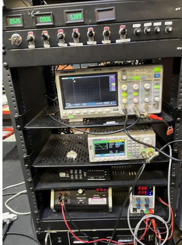
Figure 6. The rack on 2025-02-02. Top: the three gauge voltmeters (0.526, 0.906 and 5.389 V: roughing, mid-range and high-vacuum gauge outputs), the keyswitch, seven labelled toggles (Magnet, Power, RF Power, Vacuum Gauges, Diff Baffle, Diff Heat, Hi Vac Gauge) and the four fused DC-rail holders at right. Below : the SDS1202X-E, the SDG1032X, the LDG autotuner, the FB103 supply and the filament supply (2.35 A).
