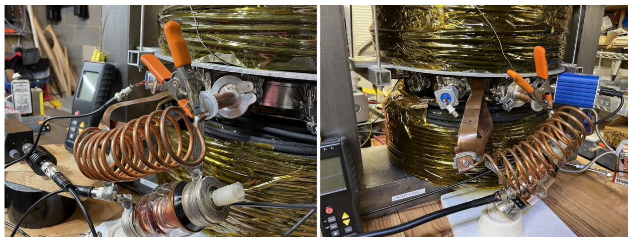
Figure 5. The matcher at port 6. Left, 2021-04-11: the bare copper tubing coil (the builder counts 11 turns) wound at the glass vacuum capacitor, whose concentric copper-cylinder electrodes show through the envelope at lower right; tinned braid runs to the copper ground strap, which disappears upward between the chamber lid and the pole; a spring clamp holds the strap to the feedthrough flange; the older UNIT mass-flow controller and the HT20 gaussmeter are in the background (media id: Live Photos/IMG_2658). Right, 2025-02-02, from the other side: the capacitor's label reads "50 nF" (50 pF, Russian surplus); the wide flat copper ground sheet runs from the feed-point braid up between the lower lid and the lower pole face; the LMR-400 feed enters at lower left on a styrofoam block; the four-pin filament/pickup feedthrough is at upper left, and "NORTH, NEG" is the pole-polarity label (media id: Live Photos/IMG_9642).
